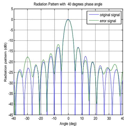
Figure 4: Effect of random error with 40<sup>0</sup> phase angle
