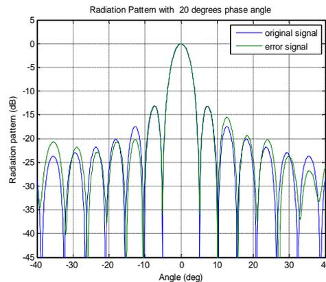
Figure 3: Effect of random error with 20<sup>0</sup> phase angle
